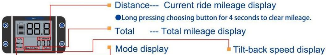
●Long pressing OK button to enter setting mode, select items which need to be adjusted then press OK to adjust items.
